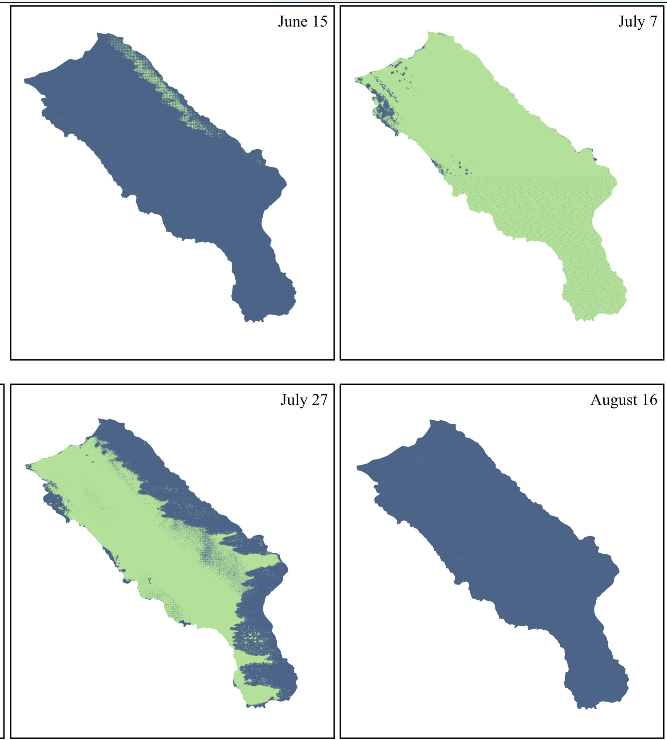
Figure 1. Cell concentrations (cells/mL) per 0.3m area classified from the random forest classification algorithm as High or Low to represent areas of Keyser Pond exceeding the NHDES threshold for cyanobacteria (70,000 cells/mL) before (June 15), during (July 7, July 20, and July 27), and after (August 16) the 2022 NHDES cyanobacteria bloom advisory.
